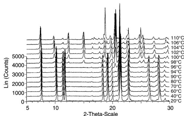
Fig. 2 Temperature-resolved XRPD analysis of the n salt.
