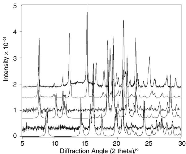
**Fig. 3** Experimental (and calculated) XRPD patterns of  $\alpha$ -methylbenzylammonium hydratropate salts. From bottom to top: p salt (calculated), p salt (exp.), n salt form I (calculated), n salt form I (exp.), n salt form II (20 °C), unstable racemic compound. The experimental patterns of p salt and n salt form I were performed with the capillary set-up in order to avoid strong preferential orientation effects.
