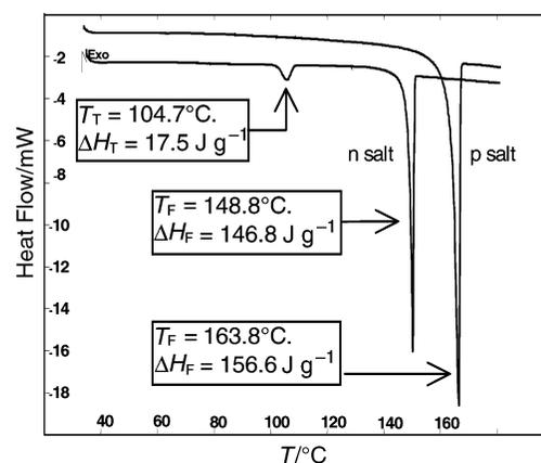
Fig. 1 DSC analyses of n salt [(+)-1-(−)-2] and p salt [(+)-1-(+)-2]. Heating rate: 2 °C min<sup>-1</sup>.
